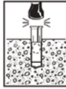
Drive Anchor flush w/surface
