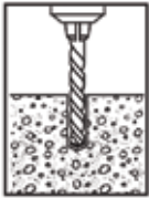
Drill hole to required depth
